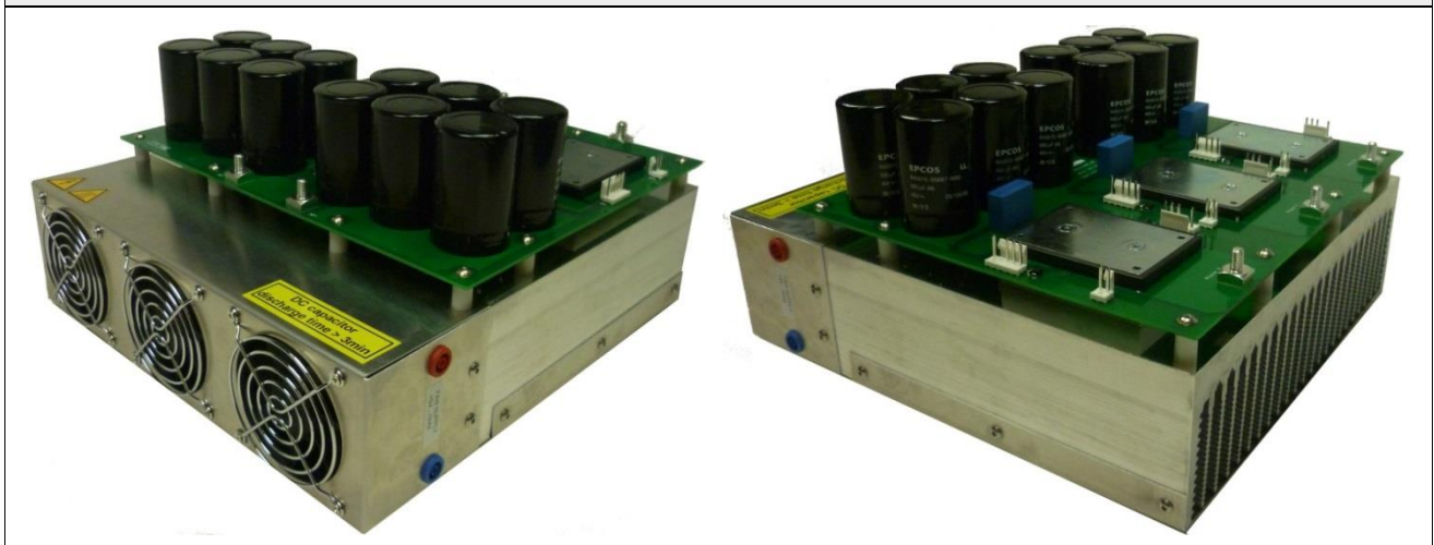
Figure 9: DC side view (left) and AC side view (right) of the 3-phase inverter
