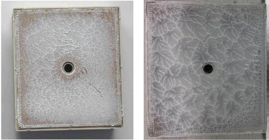
Figure 25: Correct distribution of paste (L) and too much paste (R)
